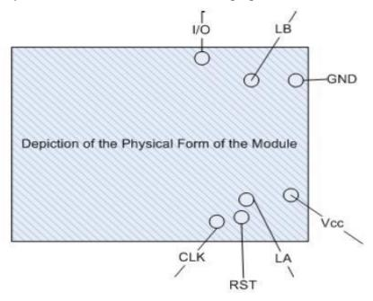
Figure 1 TOE's Physical form factor and interfaces
